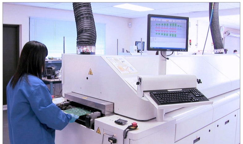
Figure 1. A printed circuit board is placed into the solder reflow oven.
