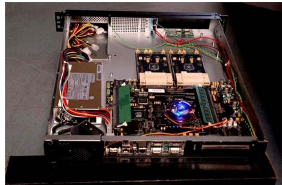
**Figure 2. ROACH board shown in 1.3 U ATX-compatible enclosure on 19" rack mount**
