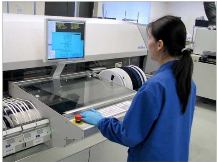
Digicom Electronics’ component placement process is geared toward flexibility, fast changeover, quick setup, and excellent accuracy and repeatability. Photo courtesy of Digicom Electronics.
