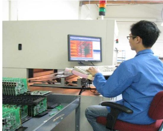
**Figure 3: Digicom Electronics' optical inspection process shown here was validated to identify the correct part and its placement**
